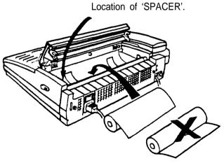
Note: If you are using 210 mm wide paper, rotate down the black 'SPACER' located in the paper compartment to fit the width of the paper roll.
